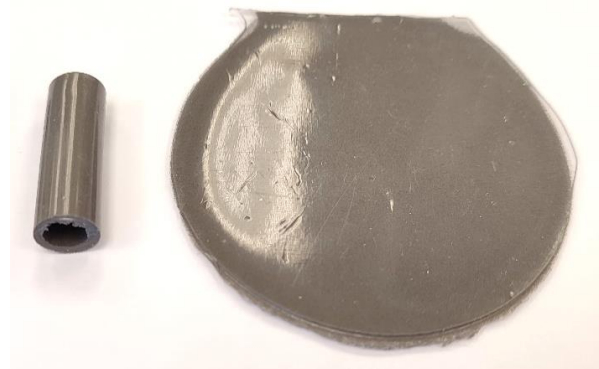
Figure 2. Magnetoactive samples of different geometry. On the left tube shape sample, and on the right elastomer layer.
