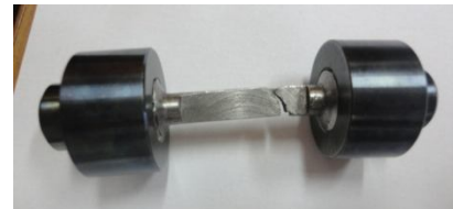
Fig.6 Specimen fractured ( T = 18^\circ\text{C} , \Delta\varepsilon = 0.5\% , f = 10 Hz, N_f = 11494 cycles).
