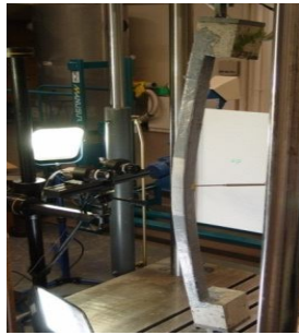
Figure 23 : Column during test.
