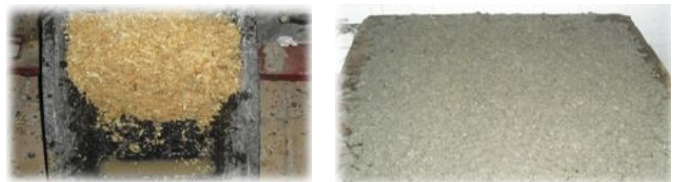
Figures 2: a) Wooden shavings after wetting.
