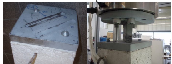
Figure 22 Load reception plate & application of the load to the top of the column
