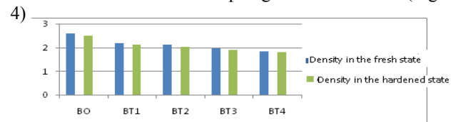
Figure 4: Change in the density of concrete with treated wood chips.
