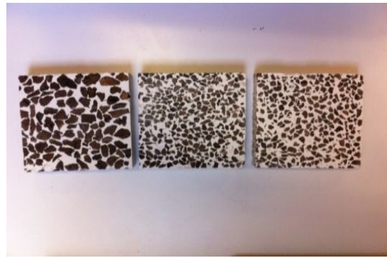
Fig.3: View of consolidated material (Plaster + Granular cork)
